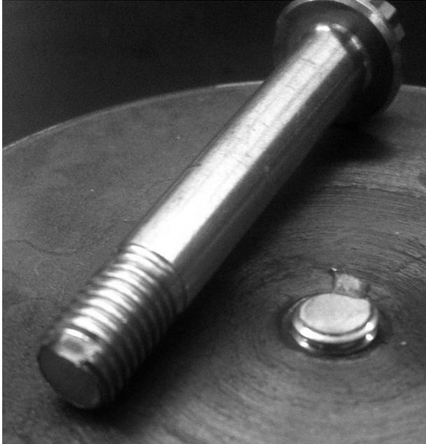
**Figure 6. Sample Ti 6-4 test fastener failure**
