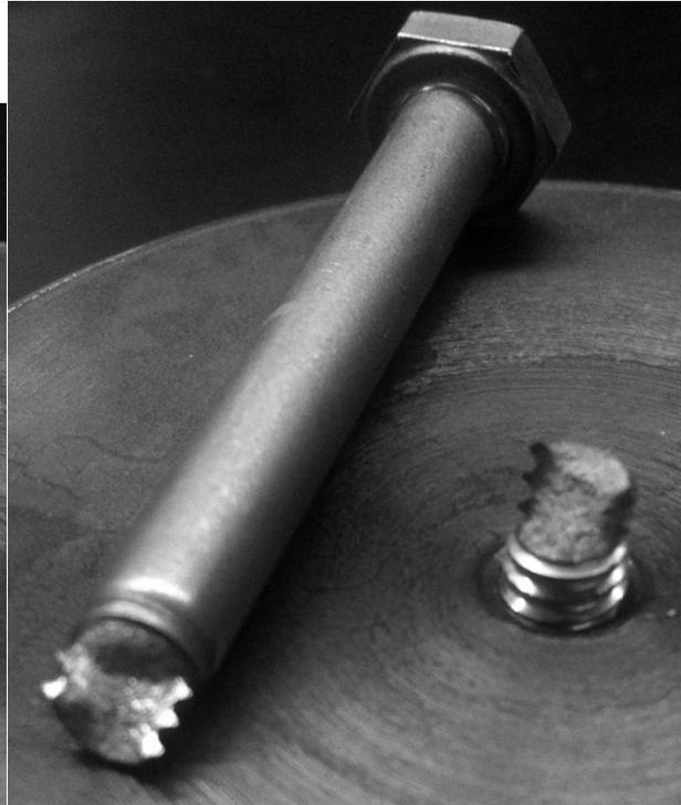
**Figure 7. Sample A286 test fastener failure**
